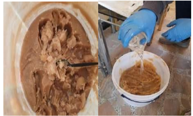
Fig (2): The mixing of paraffin wax with paraffin oil.
